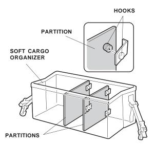
3. Place the organizer in the cargo area of the vehicle. Attach the outer hooks of the organizer to the vehicle tie-down hooks.
